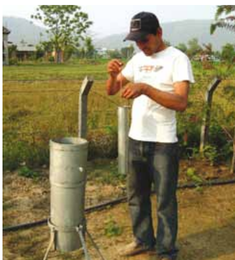
Photo 11: Measuring rain water by ruler.
