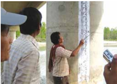
Photo 7: Gauge painted on bridge pillar
