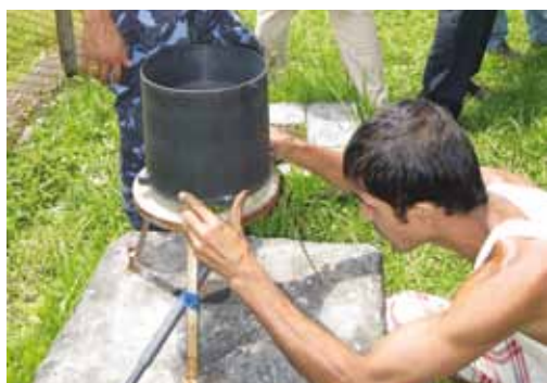
Photo 10: Automatic tipping bucket.
