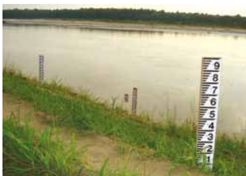
Photo 9: Water level gauges.
